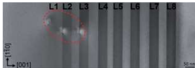
Figure W4.1.7. Bright-field g=004 TEM image of the UPM multi-layer structure examined by ESR6 and ESR7 at UOW. The dark layers are GaAsSb while the lighter layers are GaAs. Dislocations at the interface of L1-L3 are highlighted by the dashed red oval.
